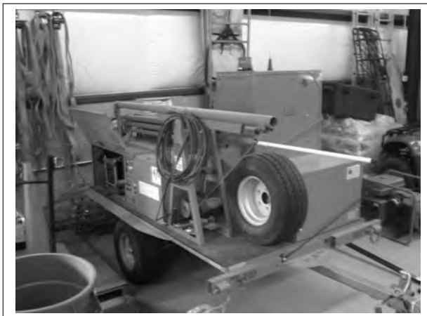
Figure 11.1. A trailer-mounted portable repeater unit
