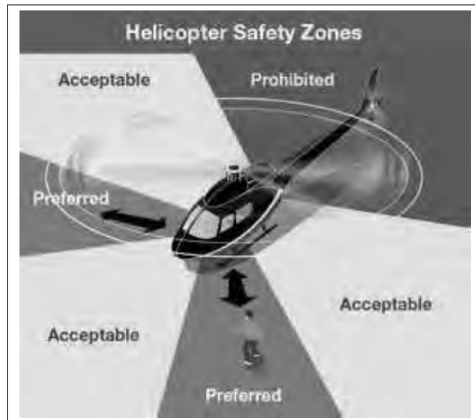
Figure 5.2. Helicopter safety zones
